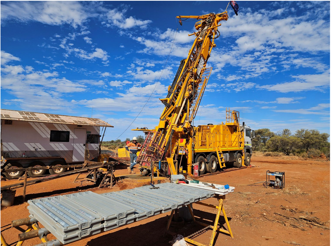
Photo 1 : DDH1 Diamond Drill Rig in operation at Yundamindra Gold Project.
